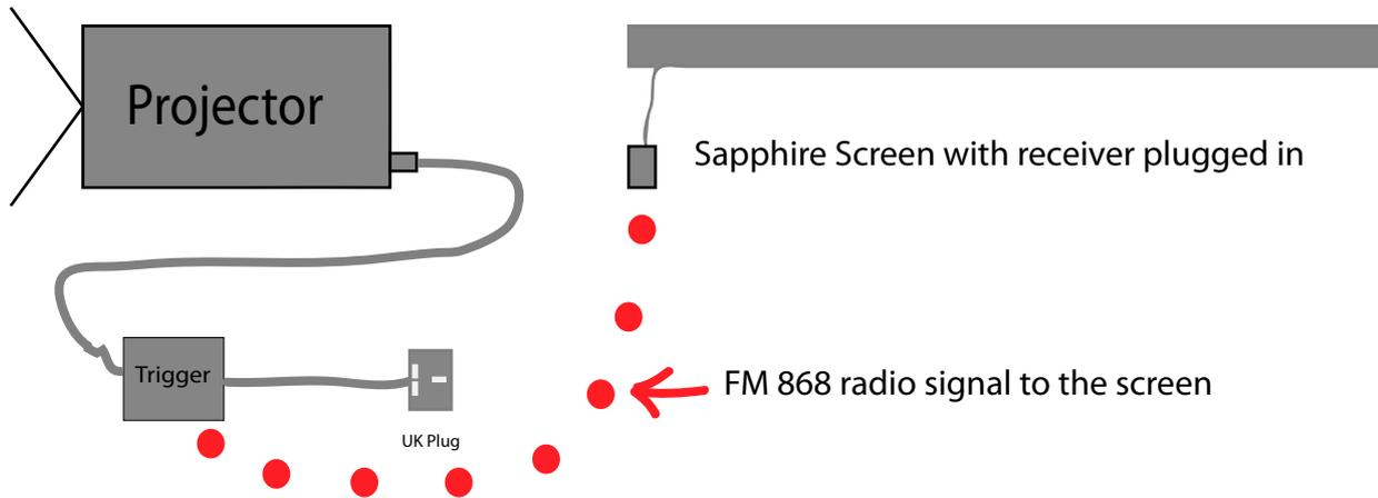
The **STR12v** unit for projectors with 12v out - sender unit and connecting to a projector
